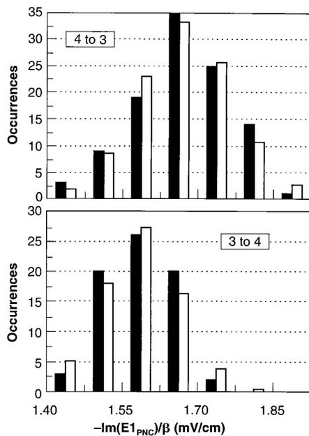
**Fig. 3.** Histograms of 1.5 hour blocks of PNC results for the  $6S_{F=3}$  to  $7S_{F=4}$  and the  $6S_{F=4}$  to  $7S_{F=3}$  transitions. The solid bars are the data, and the open bars are the theoretical distributions expected for random samples with standard deviations matching the independently measured short-term noise in the data.
