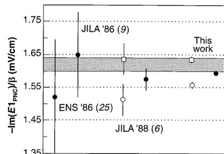
**Fig. 4.** Historical comparison of cesium PNC results. The squares are values for the 4-3 transition, the open circles are the 3-4 transition, and the solid circles are averages over the hyperfine transitions. The band is the standard-model prediction for the average, including radiative corrections. The  $\pm 1\sigma$  width shown is dominated by the uncertainty of the atomic structure.
