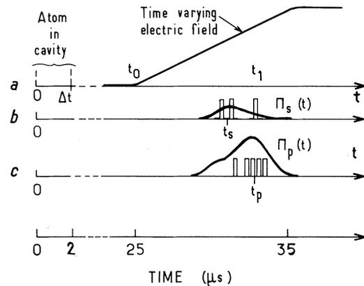
FIG. 2. Detection time sequence. *a*, Ionization field; *b*, detection of the 23S initial level; *c*, detection of the 22P final level.
