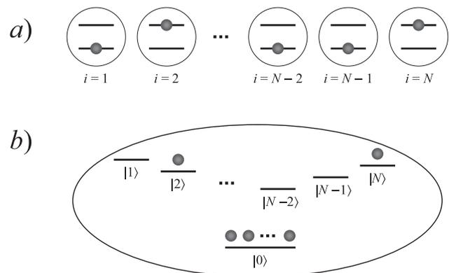
FIG. 1. Encoding of qubits in two-level and multilevel atoms. (a) Conventional qubit encoding of the  $N$ -bit state  $|01\dots001\rangle$  in  $N$  two-level systems. (b) Qubit encoding in the symmetric states of an ensemble of  $(N + 1)$ -level systems. The state  $|0\rangle$  is a reservoir state, populated initially by all atoms. Bullets represent the number of atoms populating the different single-particle states to encode the  $N$ -bit state  $|01\dots001\rangle$ .
